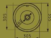
Arco Mini Single bowl Ref. 25201 £198 Overall size: Ø355 mm Bowl size: Ø305/170 mm Cutout size: Ø335 mm Minimum cab size: 350 mm Waste included: 60 mm BSW
