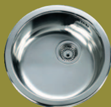
Arco Single bowl Ref. RB450B £132 Overall size: Ø440 mm Bowl size: Ø390/185 mm Cutout size: Ø416 mm Minimum cabinet size: 450 mm Waste included: 90 mm BSW
